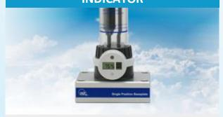
The Electronic Indicator Device progressively displays real-time consumable maintenance status instead of a 'last-minute' colour change from traditional indicators.
